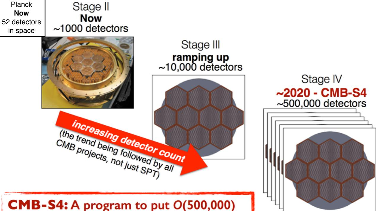
**CMB-S4:** A program to put O(500,000) detectors spanning 30 - 300 GHz using multiple telescopes and sites to map ≥70% of sky.
