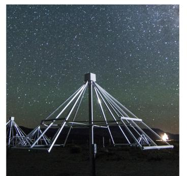
Figure 2. A picture of an LWA antenna.
