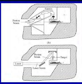
Gantries for conventional accelerator 100 tons and an optical gantry which is very compact, light using mirrors
