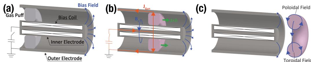
Typical CT formation process by MCPG. (a) Gas inlet (b) apply high-voltage to generate the plasma (c) accelerated plasma is captured by bias field and eject a magnetized plasmoid
