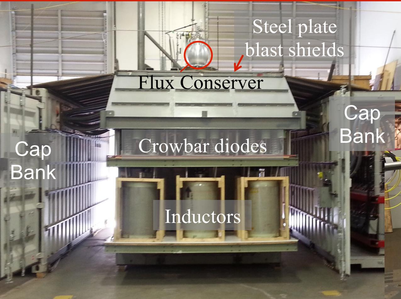
Flux Conserver only has diagnostic access on top plate to allow for uniform implosion of spherical vessel.
