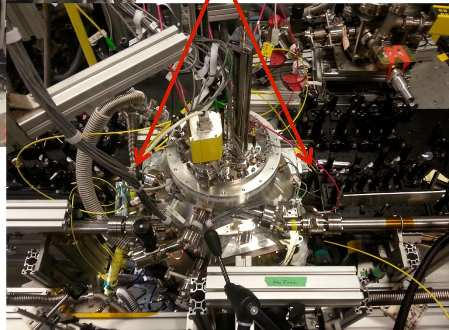
Spector 1 vessel has good diagnostic access on flux conservser.
