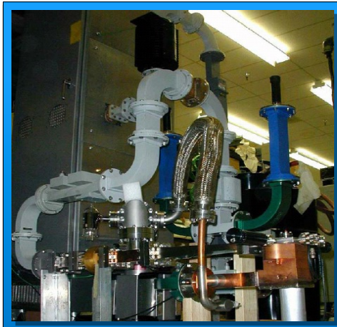
FIGURE 10. Left - S-band MPG brazed to a short 1.5 cell RF accelerator. Right- S-MPG RF accelerator installed with appropriate RF waveguide components.
