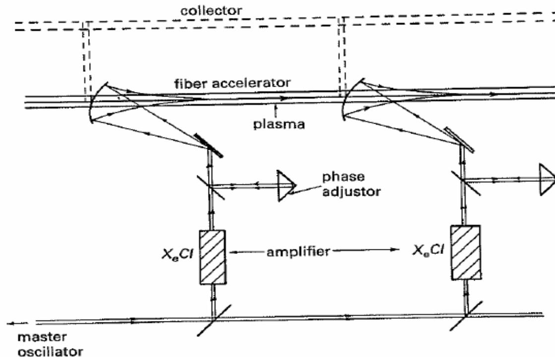
FIGURE 34. A conceptual plasma fiber accelerator with laser staging amplification *in situ*. The separation between the modules is characterized by the sum of the focal length and the pump depletion length. An example of  $X_eCl$  lasers is taken.
