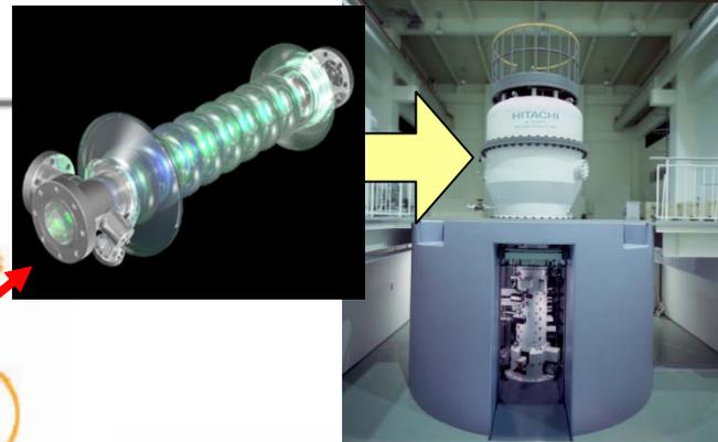
Ultra-High Voltage STEM with Superconducting RF cavity
