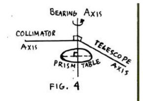
1) Spectrometer Alignment: The spectrometer must first be adjusted so that the eyepiece is focused on the crosshairs, the crosshairs are at the focal point of the telescope's objective, and the telescope axis, collimator axis and prism table are all perpendicular to the bearing (rotation) axis of the spectrometer (Fig. 4). The full procedure, using the method of autocollimation, is described in the manual for the Spencer Spectrometer; we give a shortened description here.
