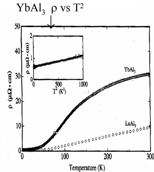
Fig. 1. Temperature dependence of the electrical resistivity of  $\text{YbAl}_3$  and  $\text{LuAl}_3$ . The inset shows the  $T^2$ -dependence of the resistivity.
