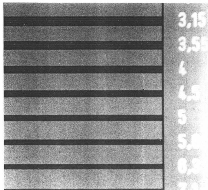
Fig. 4.13 Radiograph of a bar target illustrating phase shifts. Note that the modulation of the bars vanishes at 4.5 lp/mm, and that the phase of the modulation at lower frequencies is opposite that at the higher frequencies. (Courtesy of Meryll Frost.)
