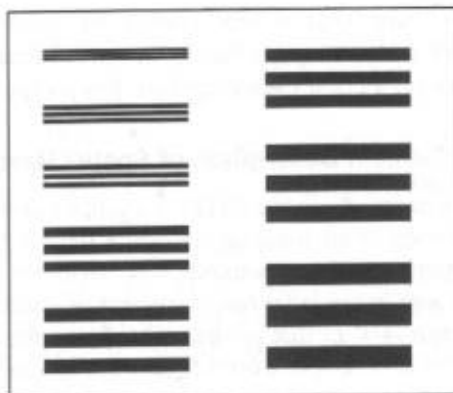
Figure 5.18. Line pair phantom. Phantoms such as this are used to measure the resolution capabilities of an imaging system in the field. This "quick and dirty" kind of measurement provides less information than an MTF, but it is a very practical way to monitor the resolution of an imaging system on a routine basis.
