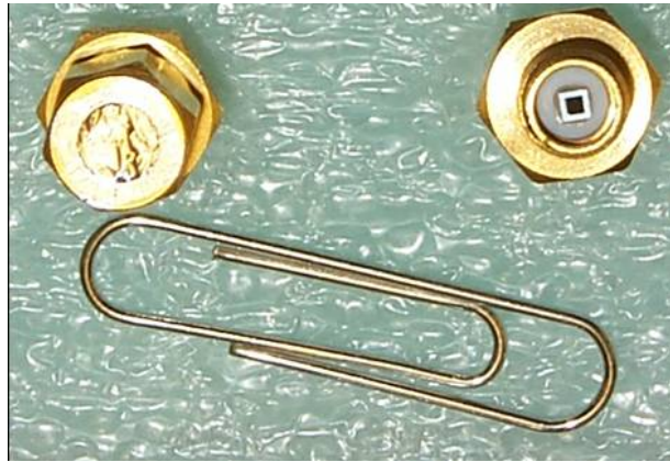
Figure 3.1: Silicon photodiodes used in the SSNPA diagnostic.
