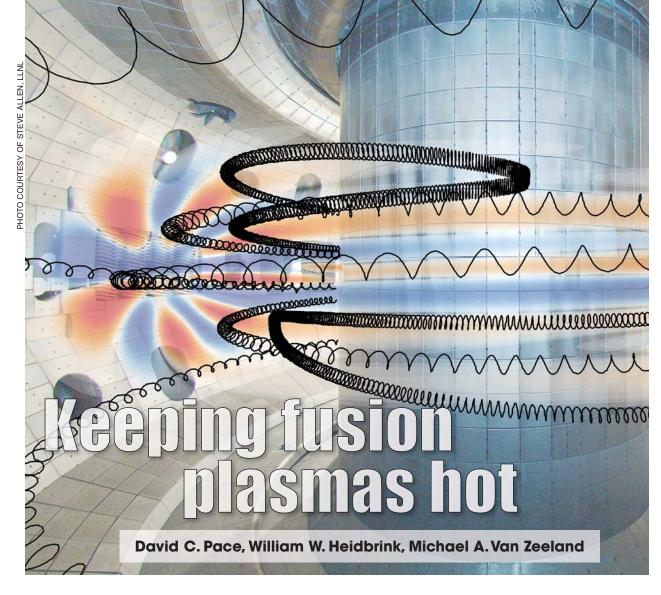
Interactions between electromagnetic waves and the most energetic ions in a plasma can perturb the orbits of those ions enough to expel them from the confining magnetic field.
