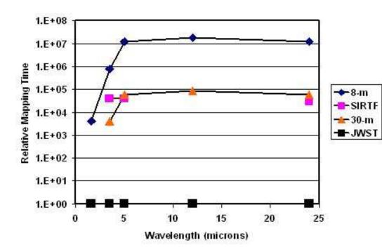
NIRCam and MIRI sensitivity complement each other, straddling  $\lambda \simeq 5 \, \mu$ m. Together, they allow objects to be found to z=15–20 in  $\sim 10^5$  sec (28 hrs).
