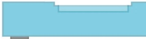
4. Align and bond two such wafers
