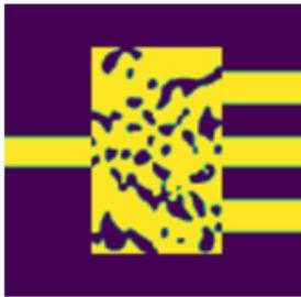
Additional development in inverse design software has allowed for integration of more advanced optimization algorithms and features to enable design of phase-controlled power splitters in 3D simulations.
