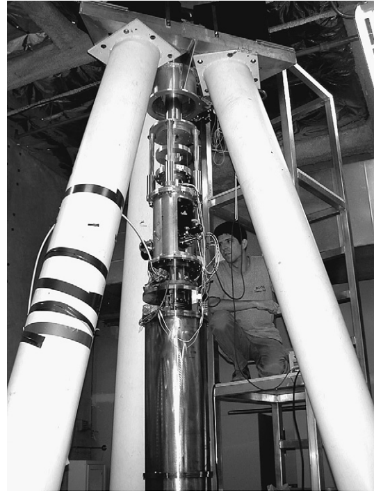
Fig. 6. Graduate student Ricco Bonicalzi adjusting room-temperature torsion pendulum apparatus in U. Washington lab (magnetic shields absent).
