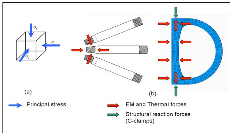
FIG. 4. "Bucking, Wedging and Bracing" structural solution for the toroidal magnet. The objective is to minimize the unbalance between the principal stress components
