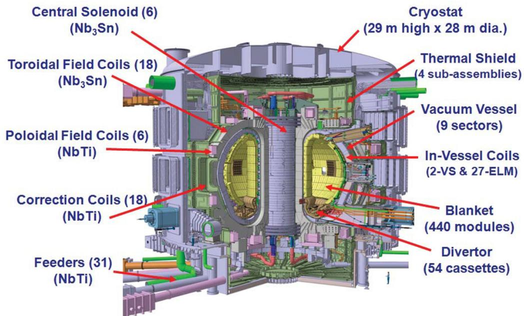
FIG. 6. Schematic diagram of the components of the ITER tokamak
