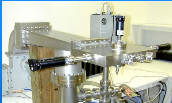
L-band experiment showing tapered waveguide and L-band MPG
