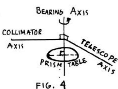
1) Spectrometer Alignment: The spectrometer must first be adjusted so that the eyepiece is focused on the crosshairs, the crosshairs are at the focal point of the telescope's objective, and the telescope axis, collimator axis and prism table are all perpendicular to the bearing (rotation) axis of the spectrometer (Fig. 4). The full procedure, using the method of autocollimation, is described in the manual for the Spencer Spectrometer; we give a shortened description here.
