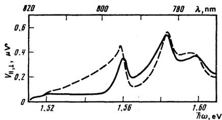
FIG. 3. Spectral dependences of the emf between the contacts in two polarizations:  $V_{\parallel}$  ( $\varphi=0$ , solid line) and  $V_{\perp}$  ( $\varphi=90^\circ$ , dashed line) in sample C52 (with allowance for normalization to the value of the photoconductivity);  $\theta=50^\circ$ ,  $T=4.2$  K.
