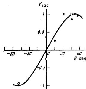
FIG. 2. Dependence of SPC on the angle of incidence of the light on the sample:  $\bullet$  sample M243,  $N\approx 7\times 10^{14} \text{ cm}^{-3}$ ;  $\circ$  sample C52,  $N\approx 5\times 10^{14} \text{ cm}^{-3}$ . The experiment and theory are normalized to unity at  $\theta=50^\circ$ . The value of  $V_{\text{SPC}}$  at  $\theta=0$  was defined as the difference between the emf when the light is polarized perpendicular and parallel to the contacts.
