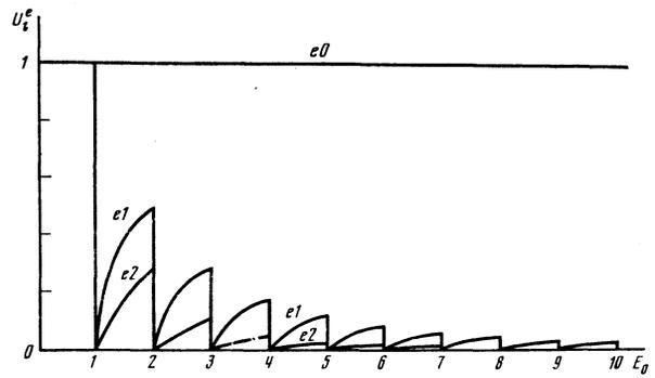
FIG. 5. Electron isotropization function  $U_l^n(E_0)$  at  $l=0, 1, 2$ . The energy  $E_0$  is marked in units of the energy of the optical phonon  $\hbar\Omega_{LO}$ . The symbols  $el$  label the plots of the functions  $U_l^n$ .
