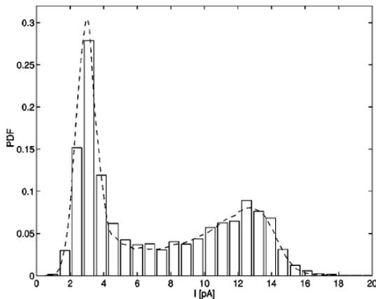
Figure 4 Histogram of ion current time series whose fragment is shown in Fig.2 (Mercik, Weron & Siwy PRE 60 (1999) 7343.
